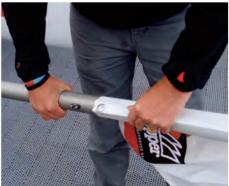
1.4 Tie the downhaul onto the pre-attached cleat on the lower mast. Pass the downhaul through the metal ring on the sail, and then back through the cleat. As shown.
