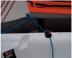
3.6A Fisherman's bend can be usedto join the two ends of the jib sheets together.
